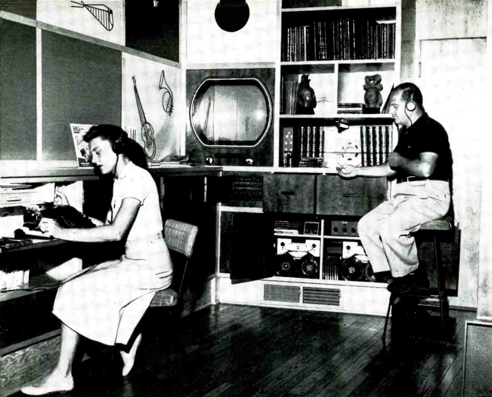
The master control unit is in the living room. Here the Schafers have three recorders running and they are set-up so they can take AM, FM or TV programs off the air. Earphones are used for monitoring each system. The "control board" is on the first shelf next to the TV set.
