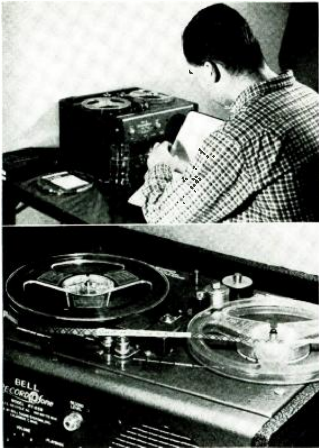
Top: the sound effects man in action. Instead of a collection of door bells, pistols, chimes, wind machines and phonograph records and a player, he has only the tape recorder and a cue sheet. As the effects have been recorded in sequence he needs only to stop the recorder between effects and he is already set-up for the next one. Lower: leader and timing tape is spliced between recordings. As a double check, the title of the effect about to pass the head is lettered on the tape. The use of the leader and timing tape also provides a check that the reel has been rewound before the next performance.
